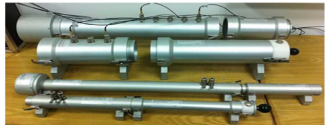
Fig. 6. Impedance tube by the transfer function method
