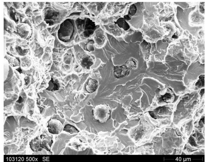
Figure 6. SEM image of fracture surface of specimen tested at 400 °C showing regions cleavage fracture (river patterns).
