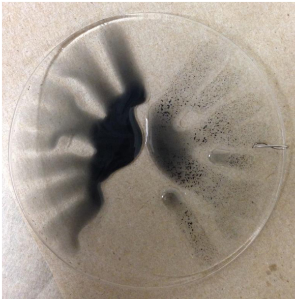
Figure 3. Droplets of 1% by weight nanoparticles (left) and microparticles (right) in oil.
