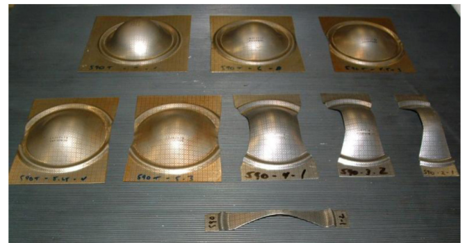
Figure 3. Samples formed using the traditional NA technique for determination of FLC
