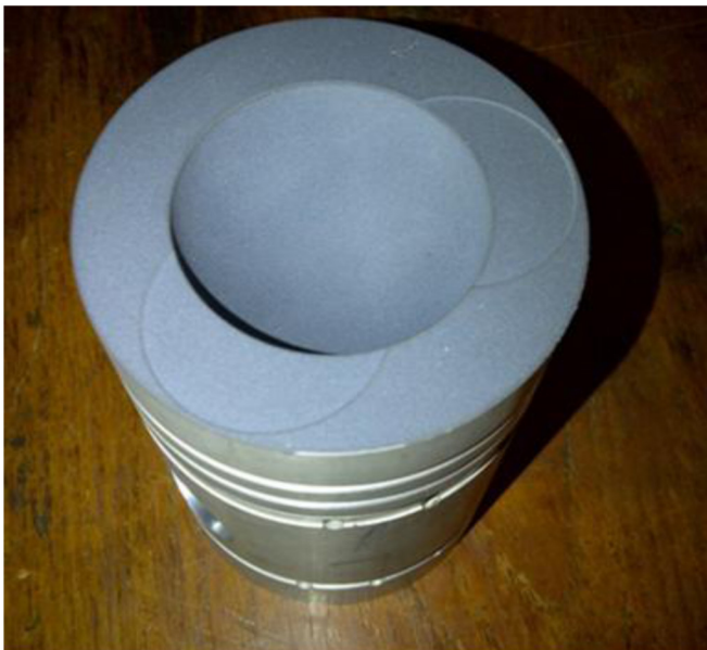
Figure 1. AV1 Diesel engine piston coated with titanium dioxide
