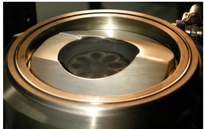
Figure 2. Picture of piston (in all-metal configuration) and cylinder in its dropped-down position.
