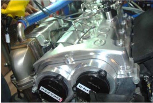
Figure 7 . Photograph of front of engine with electric phasers.
