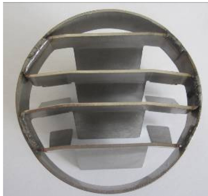
Figure 3. Mixer applied after the vaporizer
