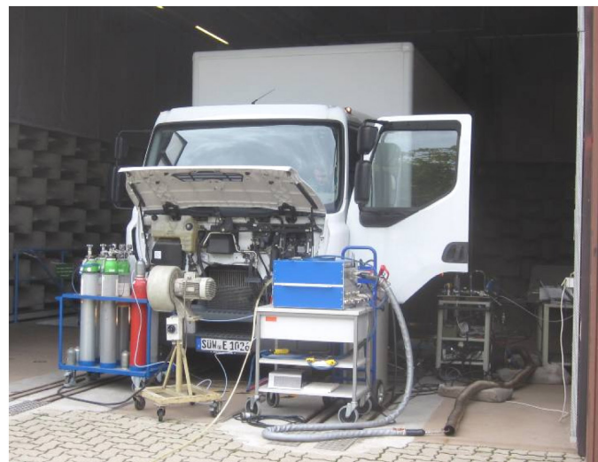
Figure 7. Chassis dynamometer experimental setup
