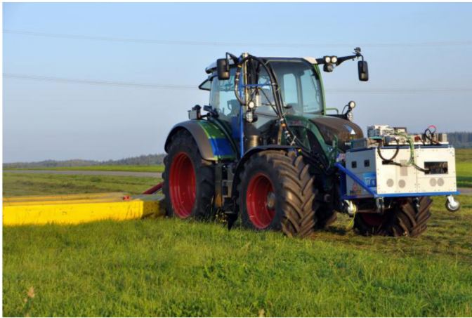
Figure 3. (cont.) Demonstrating the installation of PEMS in a light-duty vehicle (top) [39], heavy-duty vehicle (middle) [40] and non-road mobile machinery (bottom) [39].
