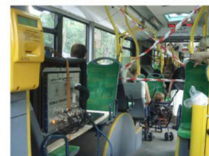
Figure 3. Demonstrating the installation of PEMS in a light-duty vehicle (top) [39], heavy-duty vehicle (middle) [40] and non-road mobile machinery (bottom) [39].
