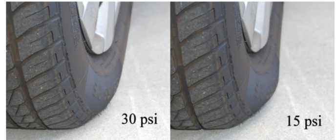
Figure 2. Toyota Corolla tire with 30psi (left) and 15psi (right).
