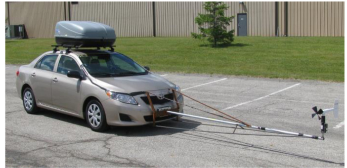
Figure 1. Toyota Corolla equipped for coast down test with a rooftop cargo box and boom.
