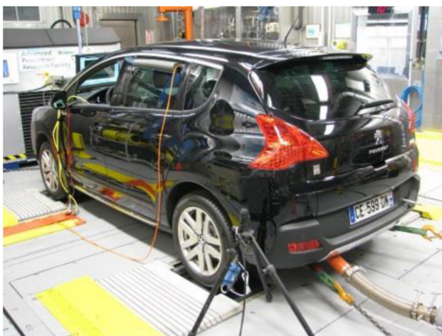
Figure 2. 3008 Hybrid4 Being Tested in Advanced Powertrain Research Facility (APRF)
