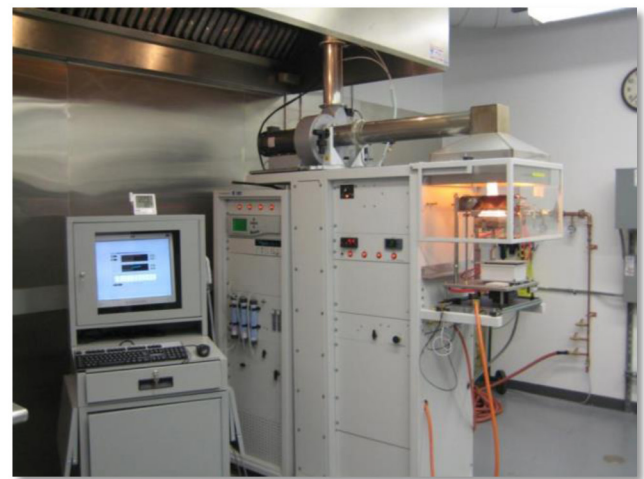
Figure 1. (a) Schematic layout of a Cone Calorimeter and (b) The Cone Calorimeter at Exponent's Bowie, MD facility.
