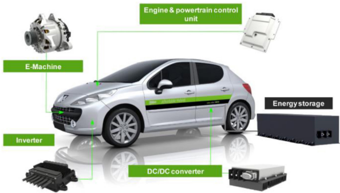
Figure 2. Components of battery electric vehicles (Hybrid4All i-BSG 48V) [6].
