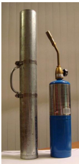
Figure 1. Experimental tube exterior and heating torch
