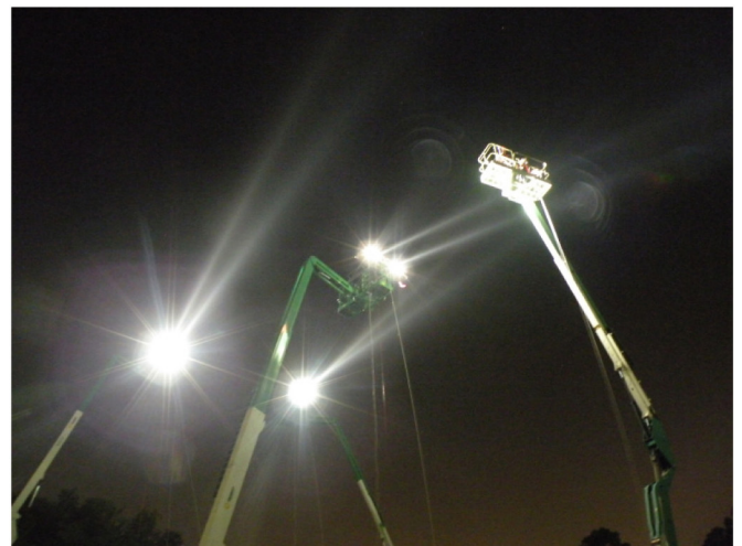
Figure 4. HID Landing Lights simulating "approach" conditions for test pilot evaluation. Fwd lift (RH side) hosting represents Flight Deck. Notice the amount of stray light illuminating this area
