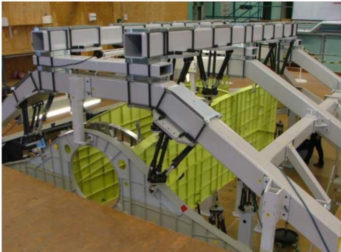
Figure 2. Reconfigurable fixture for stage one primary structures [13]
