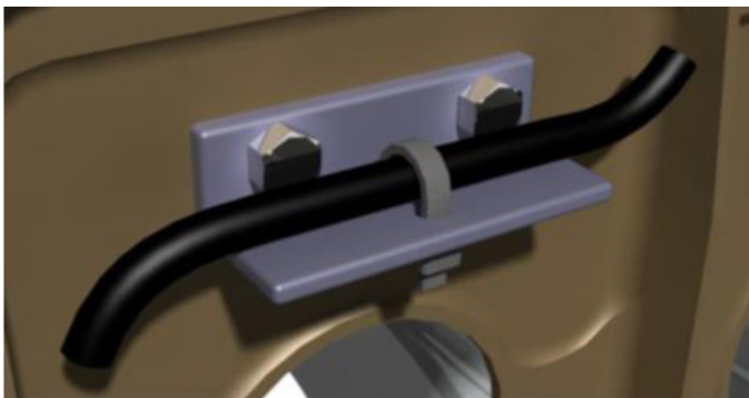
Figure 2. Bracket and cable installation existing design.
