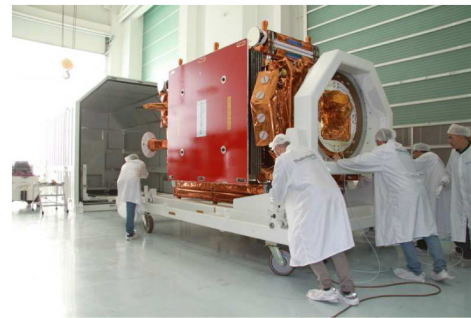
Figure 8. Satellite installation in the shipping container
