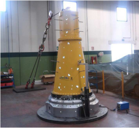
Figure 4. Marman fitting testing with a mass dummy and bending load application - photogrammetry targets.
