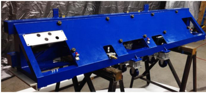
Figure 5. Machine frame rear face with aluminum "skin" prior to major machine assembly.
