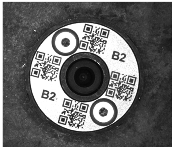
Figure 6. Floor Barcode Fiducial
