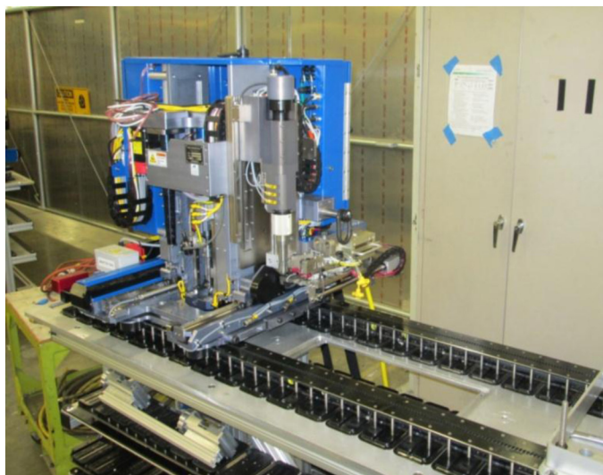
Figure 1. Electroimpact drill and fasten Flex Track for wing assembly.
