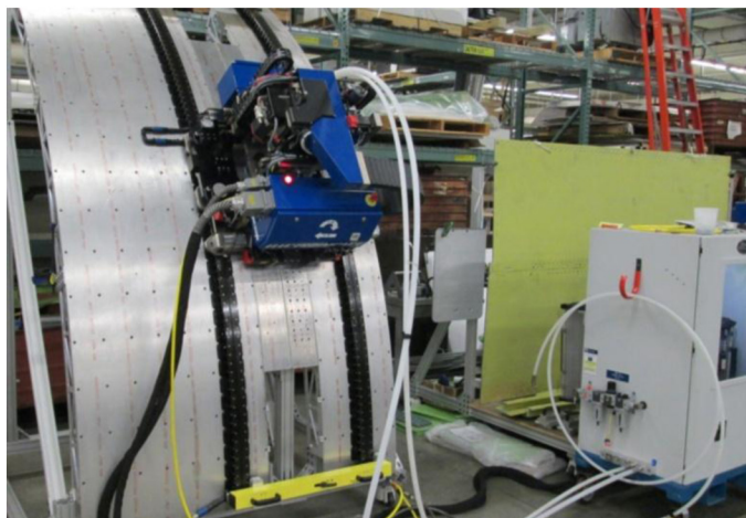
Figure 2. Electroimpact drill and fasten Flex Track with Brown aerospace fastener feed system.
