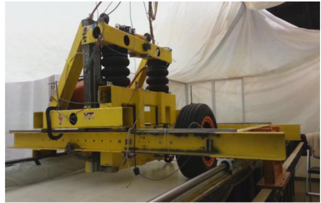
Figure 1. Terramechanics rig at the Advanced Vehicle Dynamics Laboratory, employed for study of tire-ice interactions.
