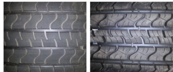
Figure 2. Tread pattern of the P225/60R 97S SRTTs tested on ice. The tire on the left has been buffed to have a tread depth of 1.6 mm and the tire on the right has full tread.
