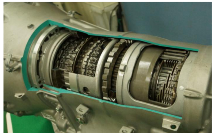
Fig.1. An automatic Transmission which consists of multiple numbers of clutch disks and clutch plates
