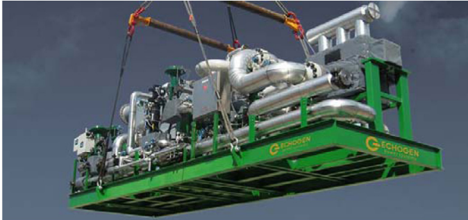
Figure 1. ECHOGEN industrial process Waste Heat Recovery System with power outputs ranging from 6MWe to 32MWe [1]. The 8MWe system has a total estimated mass of 114,000kg (Process Skid + Power Skid + Control House) [2].
