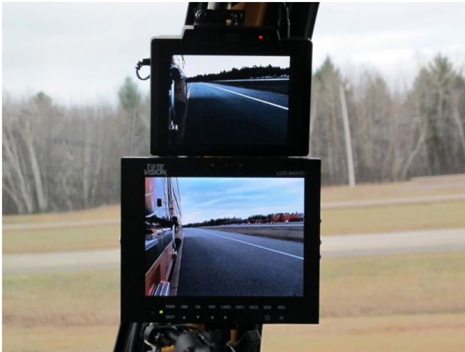
Figure 3. System monitors mounted on right A-pillar.
