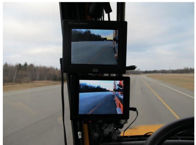
Figure 2. System monitors mounted on left A-pillar.
