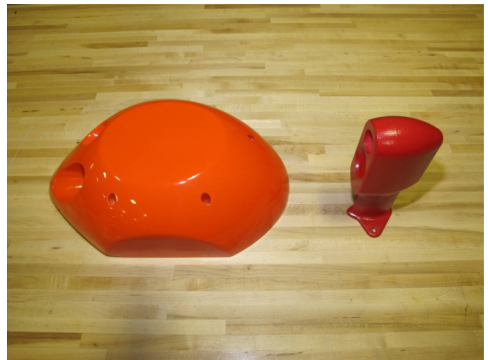
Figure 6. Camera fairings designed by NRC-AST.
