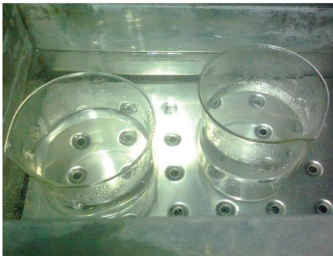
Fig 2. Treatment of Nafion membrane using peroxide bath
