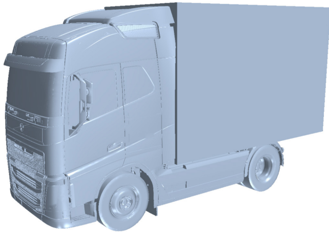
Figure 1. Vehicle geometry used for the cooling performance simulations.
