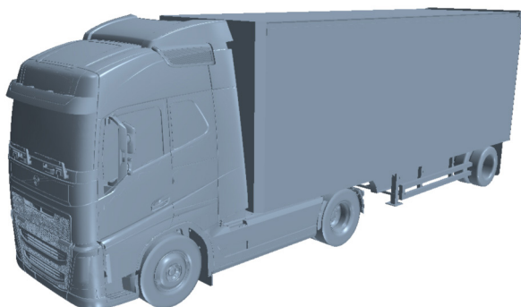
Figure 2. Geometry of the reference model for the external aerodynamics simulations.
