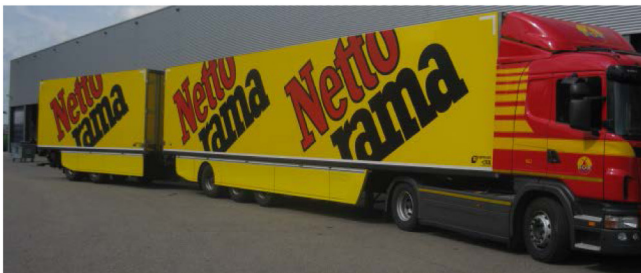
Figure 1. Illustration of the long and heavy vehicle combination: tractor semi-trailer, and a drawbar trailer.
