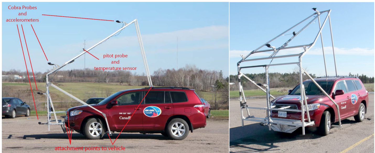
Figure 1. SUV with support rig for on-road turbulence measurements, measurement probes in vertical-array configuration.
