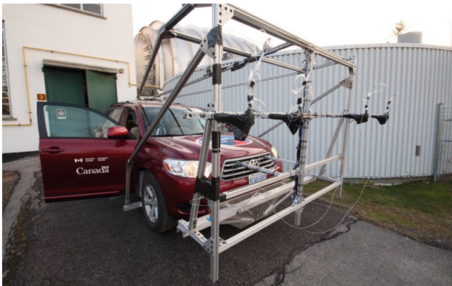
Figure 2. Horizontal probe-array configuration (with tubing system to zero the probe pressure transducers)
