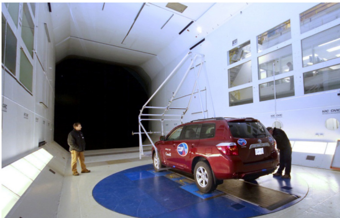
Figure 3. Test vehicle in NRC 9m Wind Tunnel
