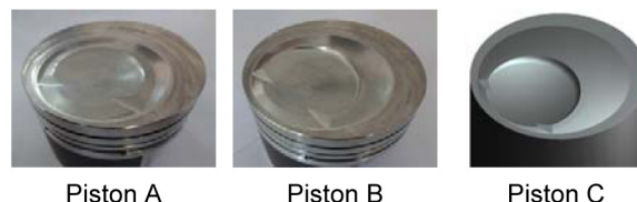
Figure 3. Newly designed bowl pistons.
