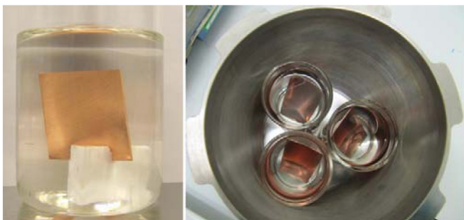
Figure 2. Exposure of Cu specimens to test fuel simulating three levels of degradation of RME (24, 48 and 72 h respectively).
