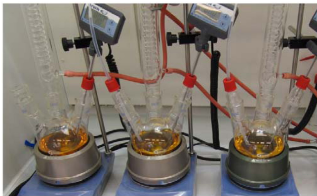
Figure 1. Exposure of Cu specimens to RME in an open system at 80°C during 24, 48 and 72 h.
