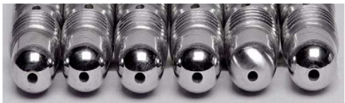
Figure 4. Passing results of the 0.4% ash - 0% phosphorus - SAE 15W-40 oil Cummins ISM injector screws.
