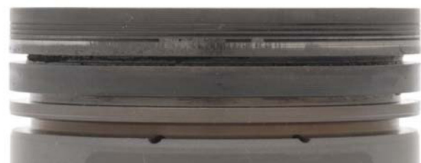
Figure 5. Passing results in the VW TDi deposit results piston/undercrown (0.4% ash - 0% phosphorus - SAE 15W-40 oil).
