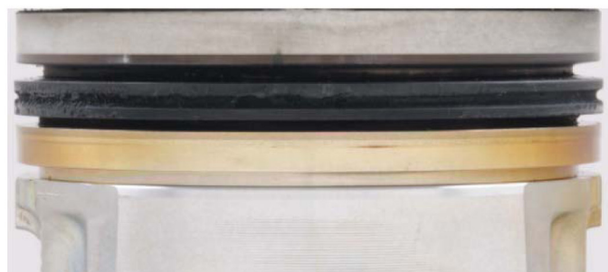
Figure 6. Passing results in Caterpillar IN (0.4% ash - 0% phosphorus - SAE 15W-40 oil).
