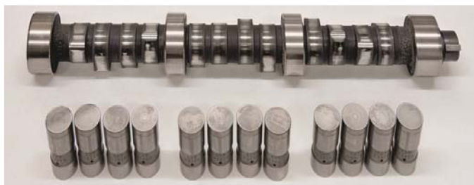
Figure 2. Passing results in the Sequence IIIG cam and lifters (0.4% ash - 0% phosphorus - SAE 15W-40 oil).
