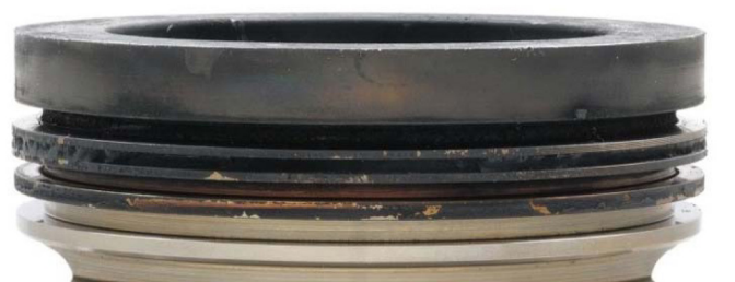
Figure 7. Passing results in Caterpillar C13 (0.4% ash - 0% phosphorus - SAE 15W-40 oil).
