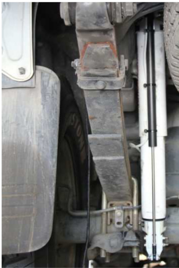
Figure 2. Toyota Hilux data logging damper and the position potentiometer attached to the left rear wheel
