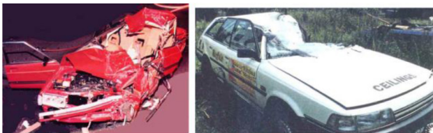
Figure 3. a. Rear end crash, b. Offset rear impact crash outcomes
