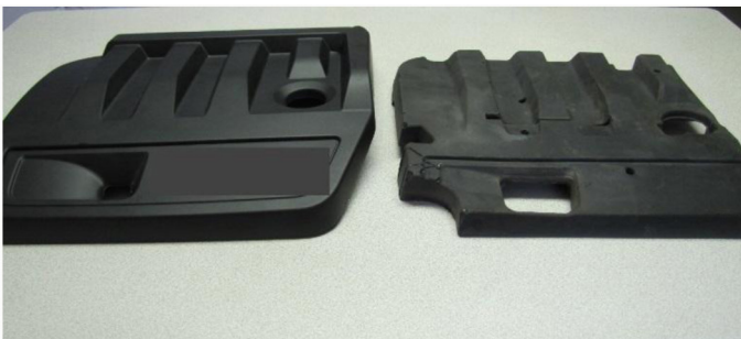
Figure 3a. Plastic cover plus polyurethane foam as insulator (side by side) (scenario 3).
