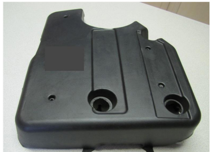
Figure 4. Painted polyurethane engine cover (scenario 4).
