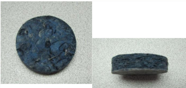
Figure 2. Shoddy material as insulator between engine and engine cover (scenario 2).
