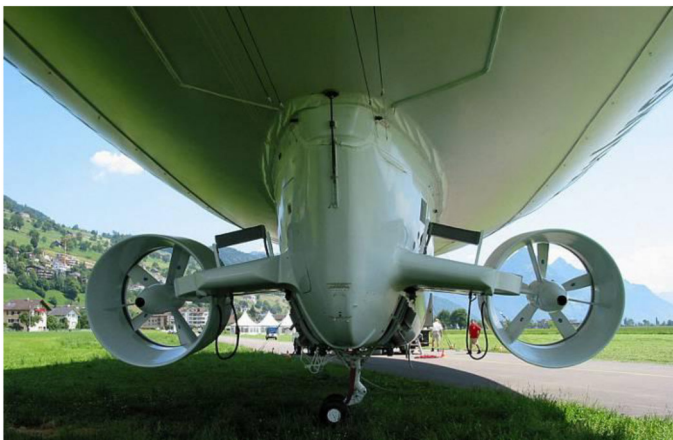
Figure 2 . Steerable ducted fans on a Skyship 600 [4]
