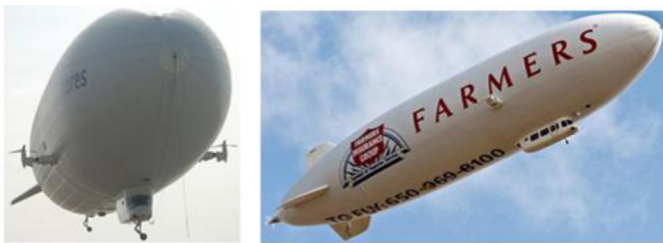
Figure 1 . Example of typical engine positions for Zeppelin-type airships [1, 3]
