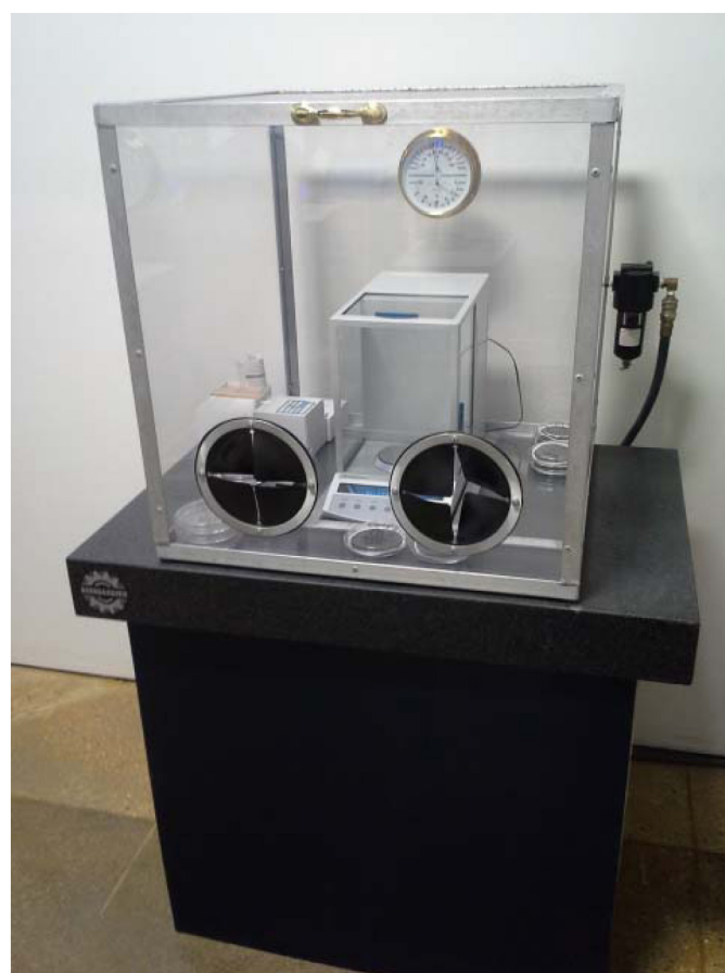
Figure 3. Constant temperature/constant humidity glove box - the scale sits atop a granite seismic mass table.
