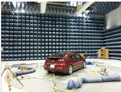
Figure 2. Vehicle level EMC test setup for a full vehicle
