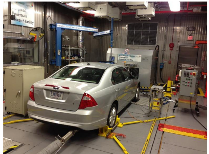
Figure 1. 2011 Ford Fusion test vehicle on APRF dynamometer for testing.
