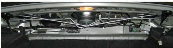
Figure 1. Typical trunk spring layout as viewed from the rear of the vehicle with the trunk open (11M Honda Civic shown).
