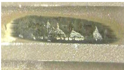
Figure 1. Peeling damage to S35C nitrocarburized gear
