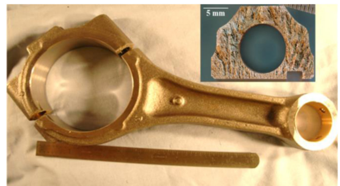
Figure 1. Example of a fracture split connecting rod with the fracture surface shown in the inset.
