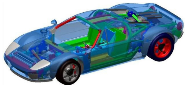
Figure 13b. Ford GT aluminum space frame.
