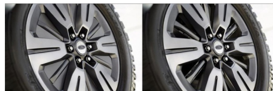
Figure 3. Active wheel shutters.
