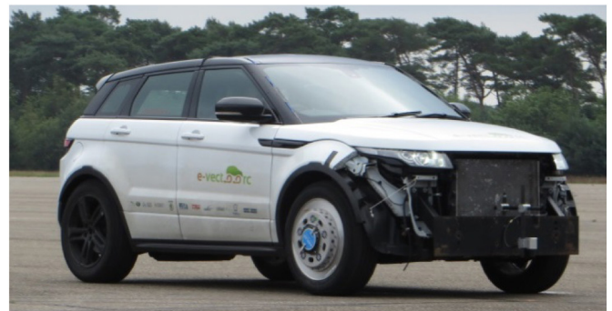
Figure 1. Range Rover Evoque equipped with four individual on-board electric motors and installed measuring hub on front right wheel
