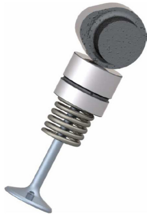
Figure 2. Direct-acting mechanical bucket tappet-type valvetrain
