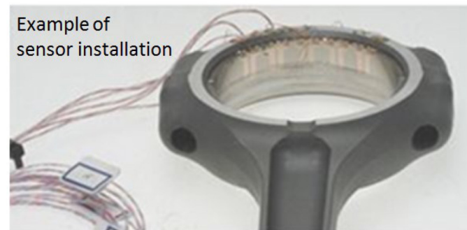
Figure 2. Thin-film sensors after testing (bearing tester)
