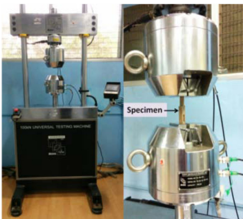
Figure 4. A servo-hydraulic UTM (on the left) with mounted specimen in close-up view (on the right)
