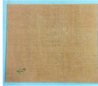
Figure 1. A jute fiber-reinforced composite laminate
