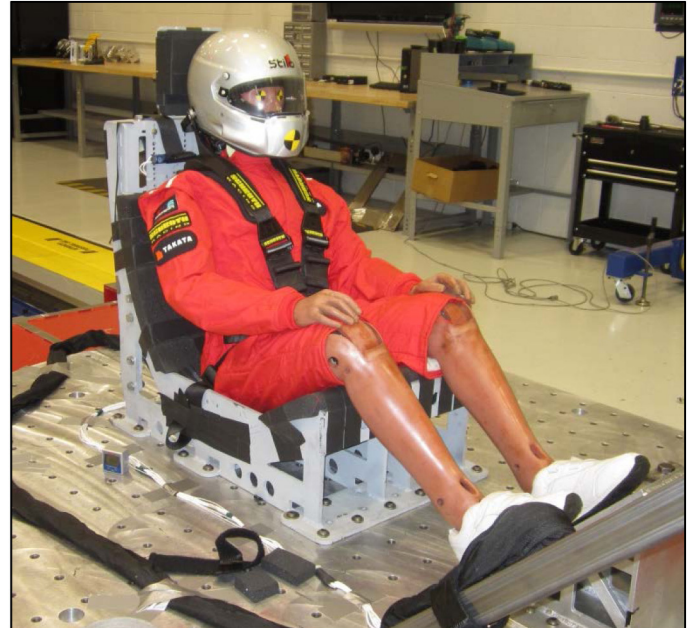
Figure 7. Sled buck with integrated shoulder belt mounts
