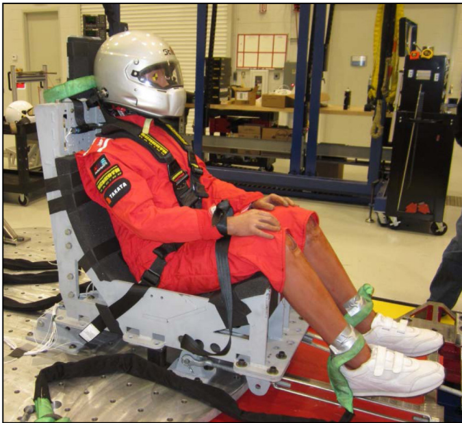
Figure 17. 50th percentile ATD positioned for vertical test, pre-rotation
