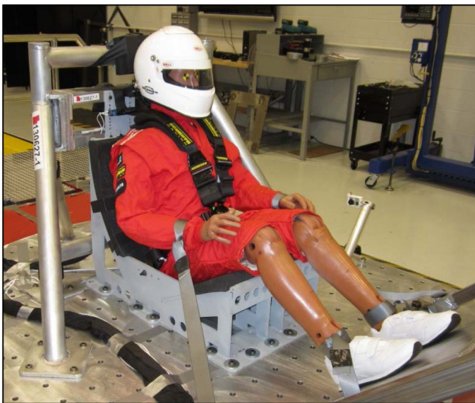
Figure 6. Sled buck with stanchion mounted shoulder belts
