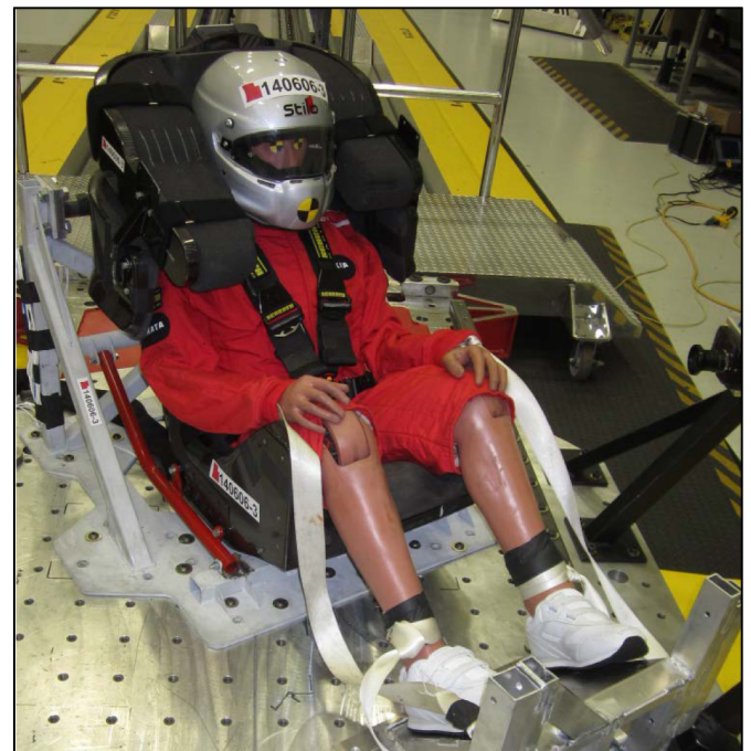
Figure 15. 50th percentile ATD 30° right frontal sled test, pre-test
