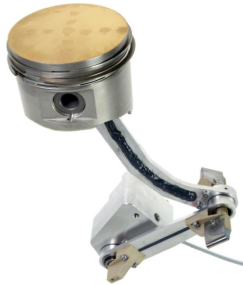
Figure 5. Piston with surface-thermocouples and assembled grasshopper-linkage.
