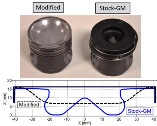
Figure 4. Stock OEM and modified piston bowl geometries for the multi-cylinder GM 1.9 L engine. The modified piston bowl was used for the present research.
